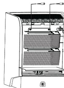
2. Insert the two thumbscrews and tighten. Insert the ActivePure Cell Assemblies connector into the plug at the rear of the unit.
