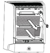
4. Slide the ActivePure Cell Assemblies down and out of the unit.
