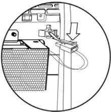
1. Unlock the ActivePure Cell Assemblies connector by pressing on the connector's locking tabs.
