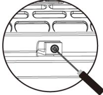
4. Use the included screwdriver to unscrew the Filter Assembly
