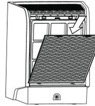
6. Replace the Back Cover by inserting the bottom in first and snapping it into place.
