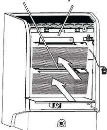
1. Insert the ActivePure Cell Assemblies up and into the unit. Position the bottom v-groove onto the center tab below and rotate up to place the top bracket onto the (2) screws located above.
