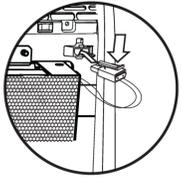
3. Press the connector firmly until the two tabs lock into place.
